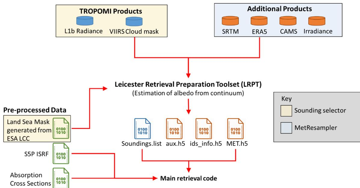
**Figure 2-1: Workflow for data inputs used within the UoL-FP algorithm for the retrieval of water vapour isotopologues from the TROPOMI instrument on board Sentinel 5P. Datasets handled by the sounding selector and MetResampler modules of the LRPT are identified with coloured boxes.**
